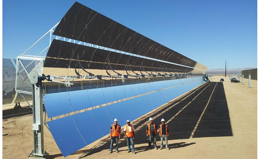
Ultimate Trough Testloop in California, USA UT deployed in Doha, Saudi Arabia
