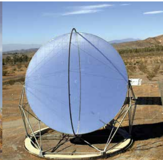
先进的膜吸定日镜 ASM 150, 150 m 2 的聚光面积 Advanced Stressed Membrane heliostat, 150 m 2 concentrator area
